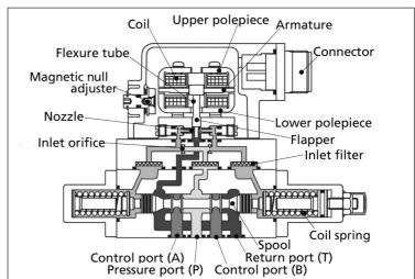
\* In summary, the spool position is proportional to the input current. With constant pressure drop across the valve, flow to the load is proportional to the spool position.
